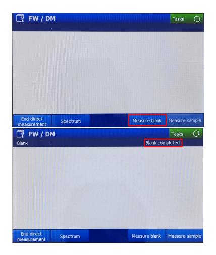
Fill the cuvette to three-fourths height with the most dilute standard. Put the cuvette to be tested into the sample pool, then click *Measure sample*, record the absorbance at 504 nm.
