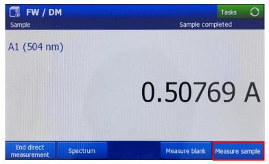
6. Then, use the next most concentrated standard to condition the cuvette. Fill it to three fourths height, click *Measure sample* and record the absorbance.
