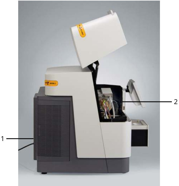
1. Electronics and support unit 2. Radiation enclosure
