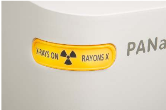
Figure 3.6 X-RAYS ON lamp on electronics and support unit
